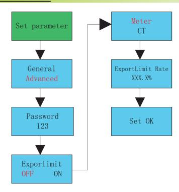
Under the permission given by your energy provider, the ratio of your system output power divided by the rated power of the inverter is called Export Limit Rate. For instance, if the energy provider only accepts 4kW from your 5KW system, then the Export Limit Rate of 5kW inverter is
