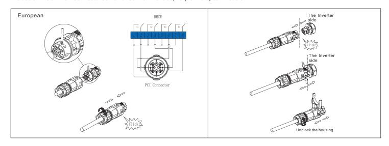
COM Port Pin Definitions- Power Control Interface (PCI).
