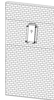
3.1.3 Put the charge point onto the bracket, and fix it with the 2 screws at the bottom of the charge point. The installation is done.
