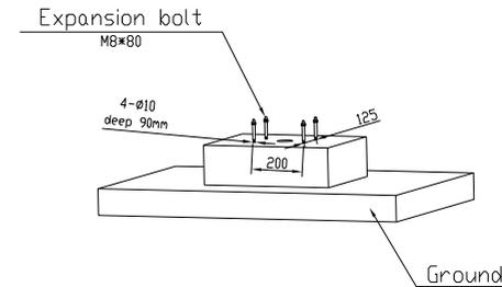
3.2.3 Fix the pole onto the holes with expansion bolts. The input cables shall go into the pole from the bottom middle area and come out of it from the area below the cable hooker.
