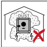
The inverter is essentially designed to be dustproof (IP 66). In areas of high dust accumulation, dust deposits may collect on the cooling surfaces, and thus impair the thermal performance. Regular cleaning is required in this case, see chapter **Operation in dusty environments** on page 117. We therefore recommend not installing the inverter in areas and environments with high dust accumulation.
